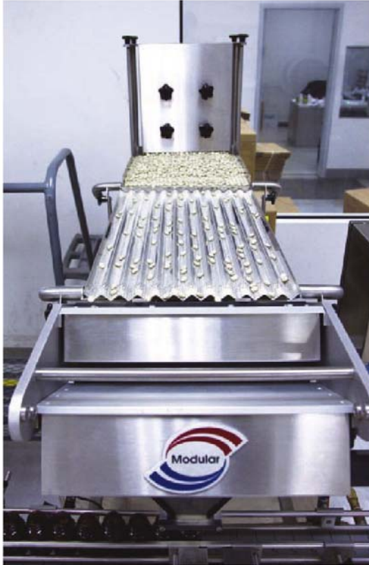
The filler uses a 12-channel system to move tablets past a sensor array, ensuring accurate counts for each bottle.
