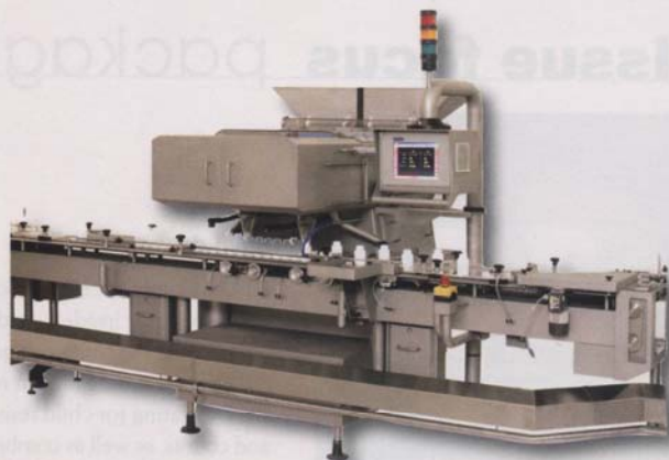
An electronic counter that uses infrared sensors [4]
